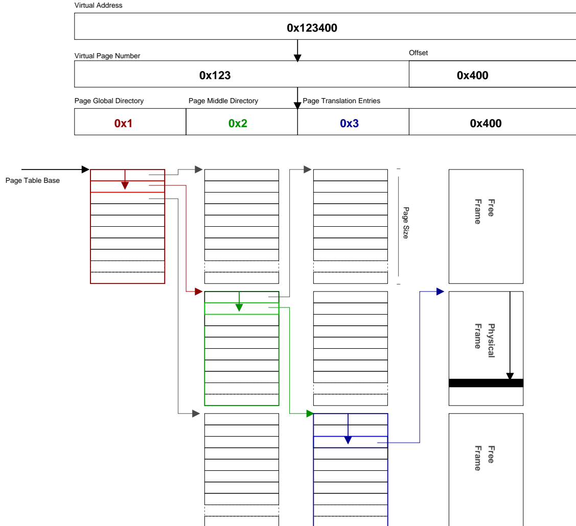
Figure 6.9. Illustration of a hierarchical page-table
